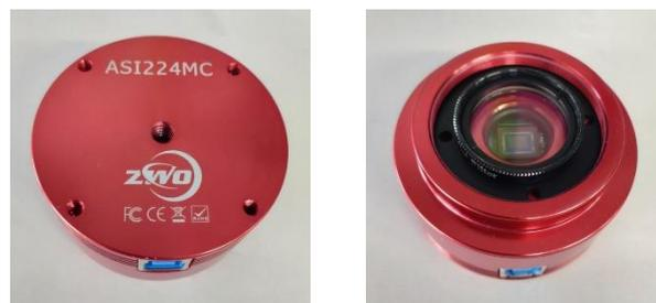
図2 CMOSカメラZWO ASI224MC
